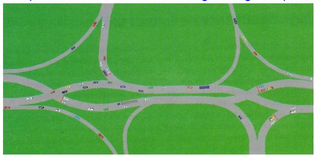
The diverging diamond interchange directs vehicle to the left side of the road to facilitate merging to and from the interstate. Traffic Signals will be placed where the arterial lanes cross and at left turns on the interstate's off-ramps.
